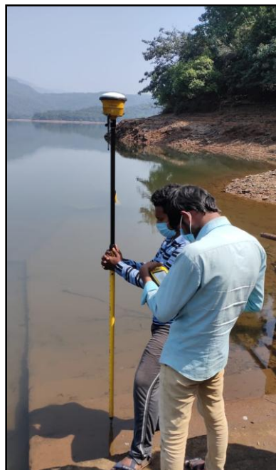
Figure 5- During Topographical Survey with RTK
